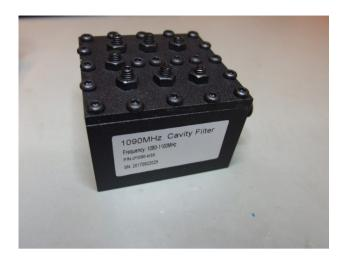
This is a cavity filter for 1090 MHz Mode-S / ADS-B.
