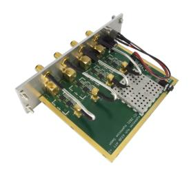
The **3U** component carrier variant is intended to be mounted in 3U high 19" component carriers conforming to IEC 60297-3-101. Such a component carrier can house a number of sysmoRFDSATT devices or other components from sysmocom (like the 16-channel GPS RF splitter) or third parties.
